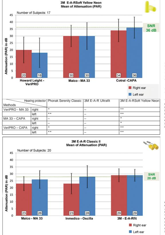
Figure 10 Comparison of PAR values for the foam earplug 3M E-A-RSoft Yellow Neon (mean values and standard deviations for 17 subjects), obtained with the measurement systems VeriPRO, MA 33 and CAPA.
