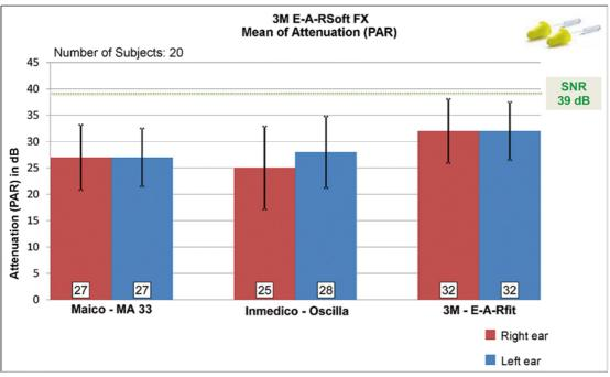
Figure 12 Comparison of PAR values for the foam earplug 3M E-A-RSoft FX (mean values and standard deviations for 17 subjects), obtained with the measurement systems MA 33, Oscilla and E-A-Rfit.
