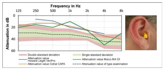
Figure 15 Comparison of the individually determined attenuation values for a subject (right ear) with the values of the type examination in the frequency range of 125 Hz to 8 kHz for the 3M E-A-R Ultrafit. The colored areas include mean ± 1 x standard deviation (light green) or mean ± 2 x standard deviation (pink). The individually determined curves are at lower attenuation values than the type examination test.
