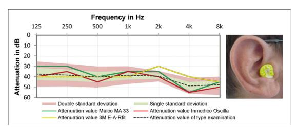
Figure 16 Comparison of the individually determined attenuation values for a subject (right ear) with the values of the type examination test in the frequency range of 125 Hz to 8 kHz for the 3M E-A-RSoft FX. The colored areas include mean ± 1 x standard deviation (light green) and mean  $\pm 2 x$ standard deviation (pink). The individually determined curves agree well with the values of the type examination test.
