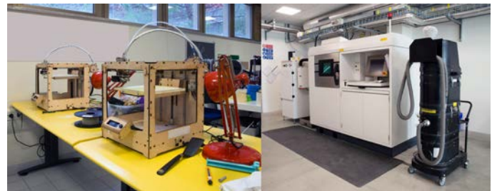
The term 3D printers covers substantially larger installations (right) as well as the relatively small desktop units (left).
