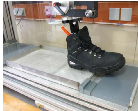
Determining the coefficient of sliding friction in accordance with DIN EN ISO 13287, method A/C – heel sliding forwards
