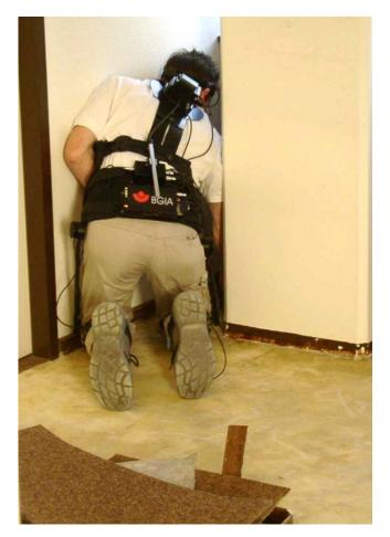
Interior decorator with the CUELA measurement system in a typical work situation: removal of old floor surfacing. Characteristics of the exposure:
