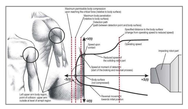
Figure 1: Kinematic process of a collision between a specific robot part and a human body; effected individual body region is the upper arm region – outside
